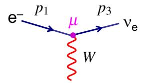
$$j^{\mu} \propto \overline{u}_{V_e} (\gamma^{\mu} - \gamma^{\mu} \gamma^5) u_e$$
